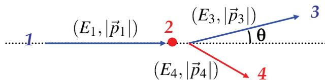
$$p_1 = (E_1, 0, 0, |\vec{p}_1|), \quad p_2 = (M, 0, 0, 0), \quad p_3 = (E_3, E_3 \sin \theta, 0, E_3 \cos \theta), \quad p_4 = (E_4, \vec{p}_4)$$
