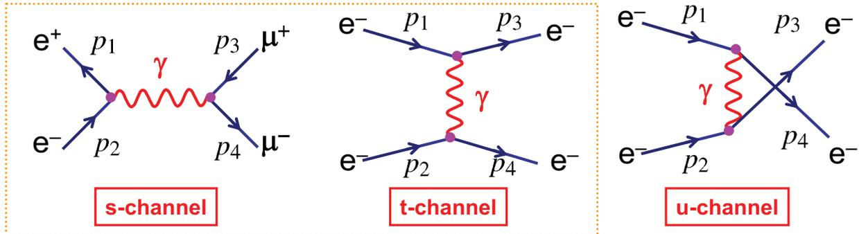
• Can define **three** kinematic variables: **s, t and u** from the following four vector scalar products (squared four-momentum of exchanged particle)
