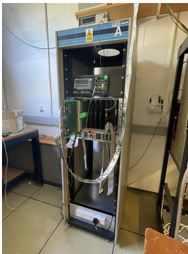
Figure 7: The data acquisition system containing all the boards. The silver strip connects to the FEBs on the RPC.
