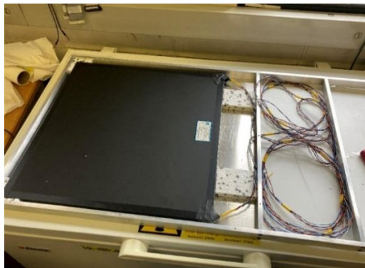
Figure 13. Picture showing how the scintillator is placed inside the metal tray, with two SiPMs in the corners. A hole on the tray allows to pass through the cables of the SiPM.
