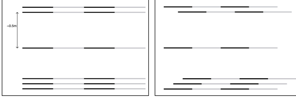
Figure 9: A schematic graph showing the parallel (Left) and off-set (Right) arrangement of RPC readout strips, with the layer separations equal to the values discussed above. All black and grey line segments represent identical RPC readout strips, the colour difference is just to make neighbouring strips distinguishable from each other. This graph is not to scale.
