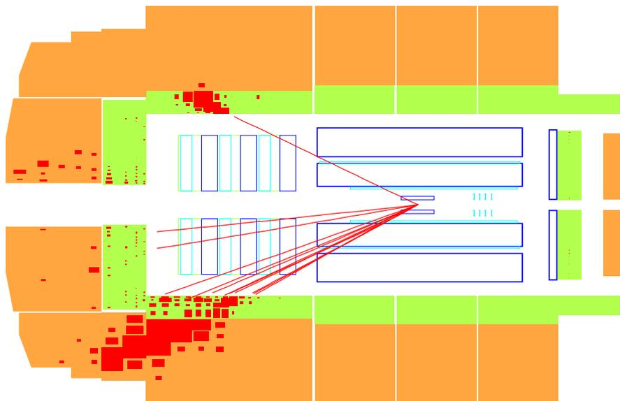
The isolated particle in the upper part of the diagram is the scattered positron, with a large signal in the electromagnetic calorimeter followed by a negligible signal in the hadronic calorimeter.
