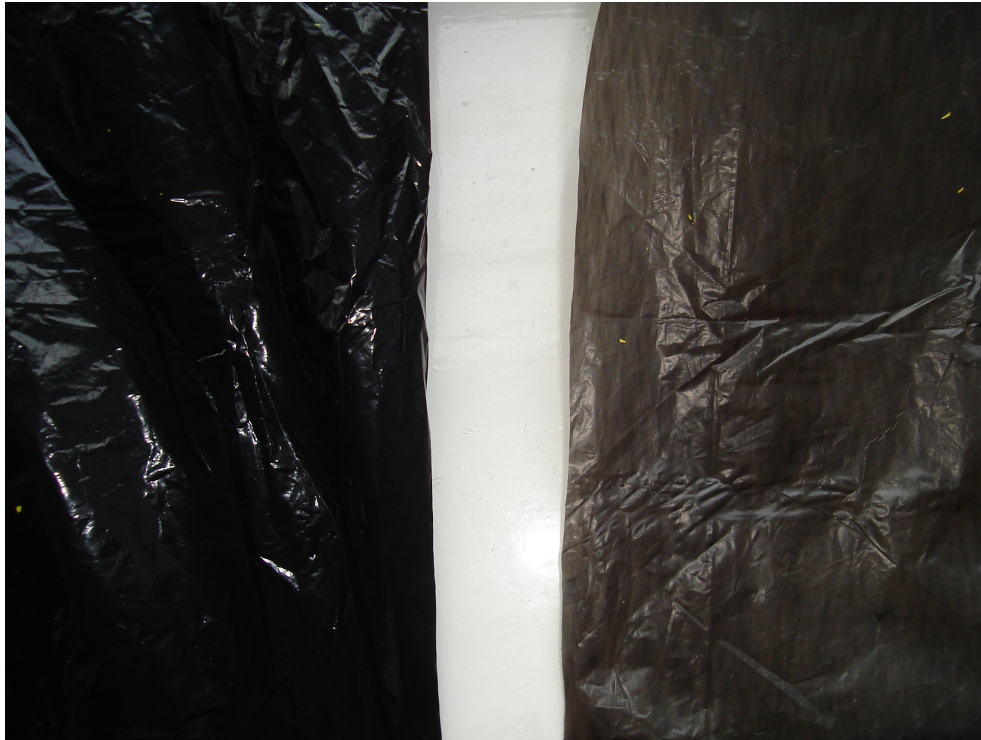
Fig 4.4 – photograph showing the colours of the solar balloon (left), and value black bin liner (right) materials. Both materials are roughly the same thickness, but the solar balloon absorbs more light due to its darker colour.
