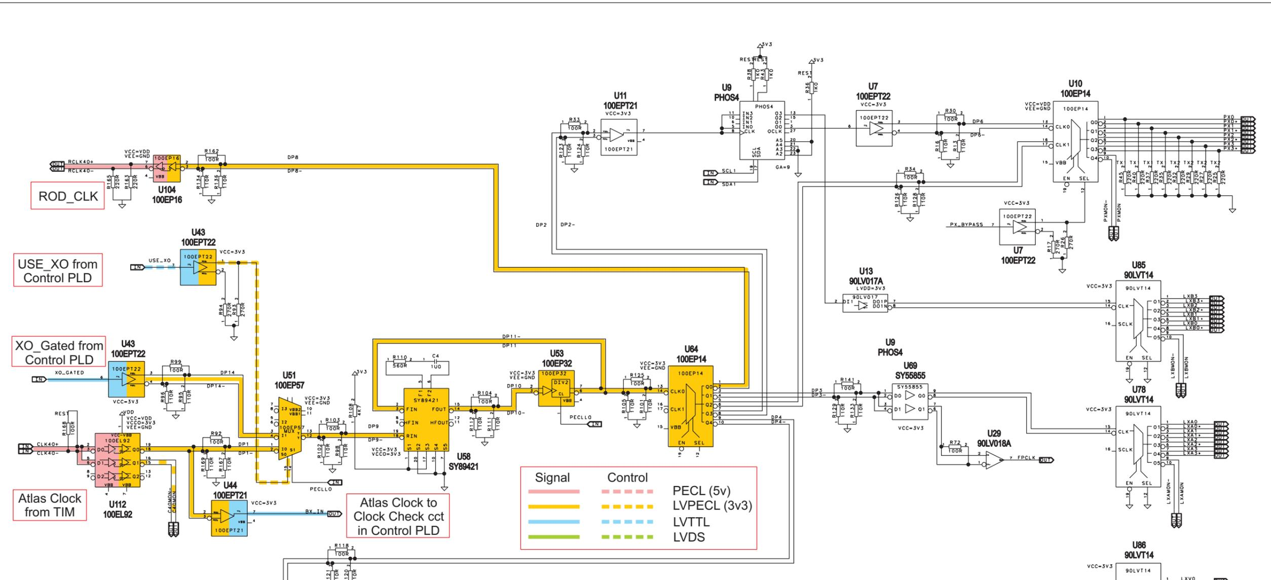
**BOC1 Revised Clock Circuits: the Central Core**
