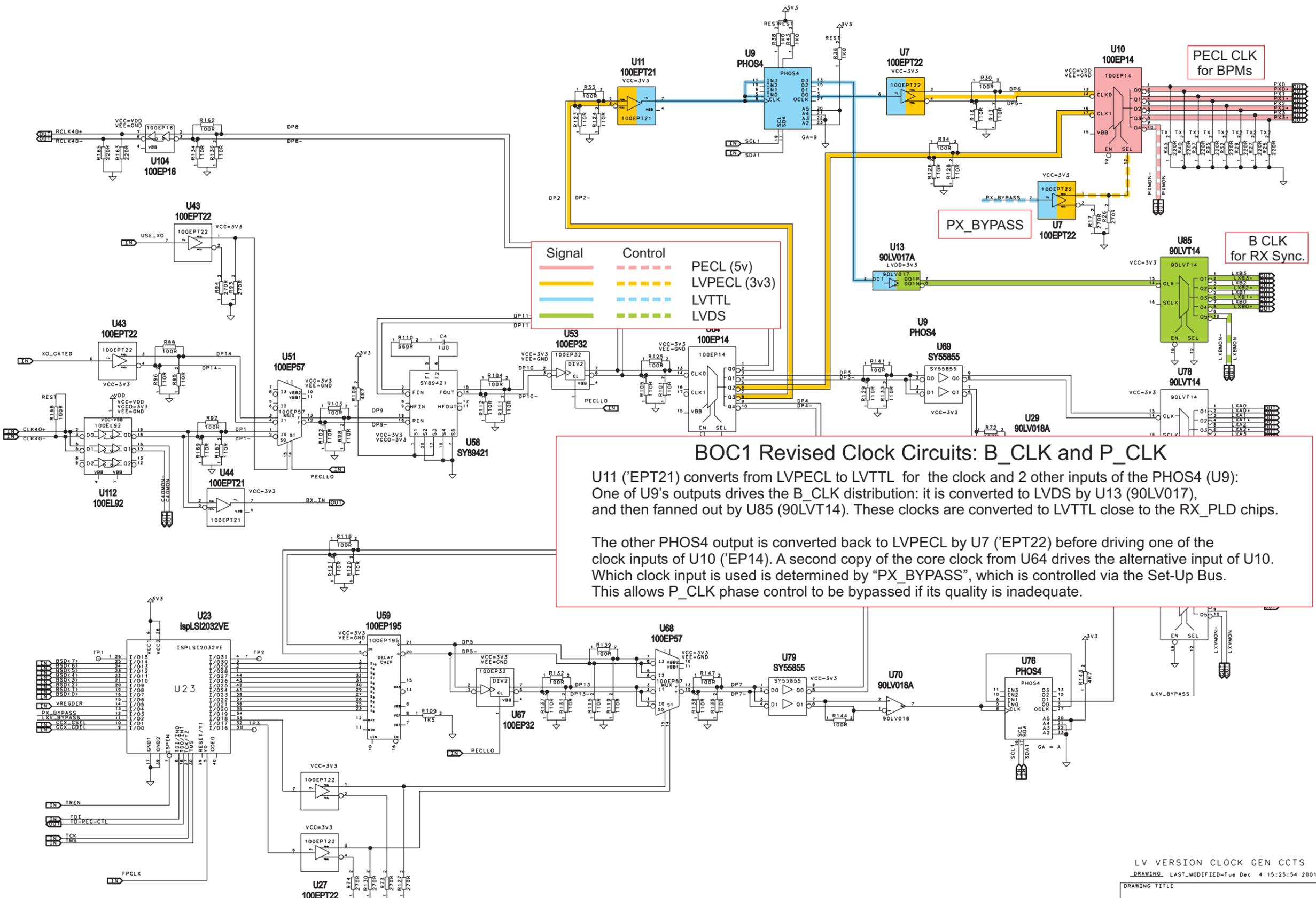
**BOC1 Revised Clock Circuits: B\_CLK and P\_CLK**
