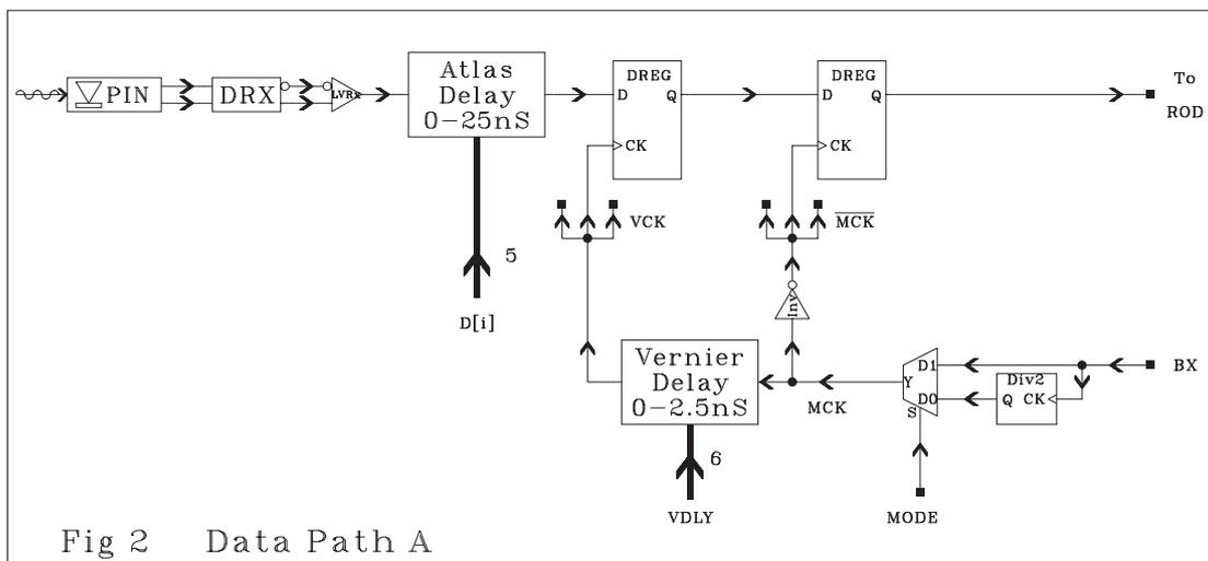
2.2.2. For each data stream the PIN diode is closely coupled to a stream of the DRX receiver chip. Its LVDS output is converted to TTL, and is then delayed by up to 25nS in 1nS steps. The delayed output is clocked into a register using a common clock VCK. The
