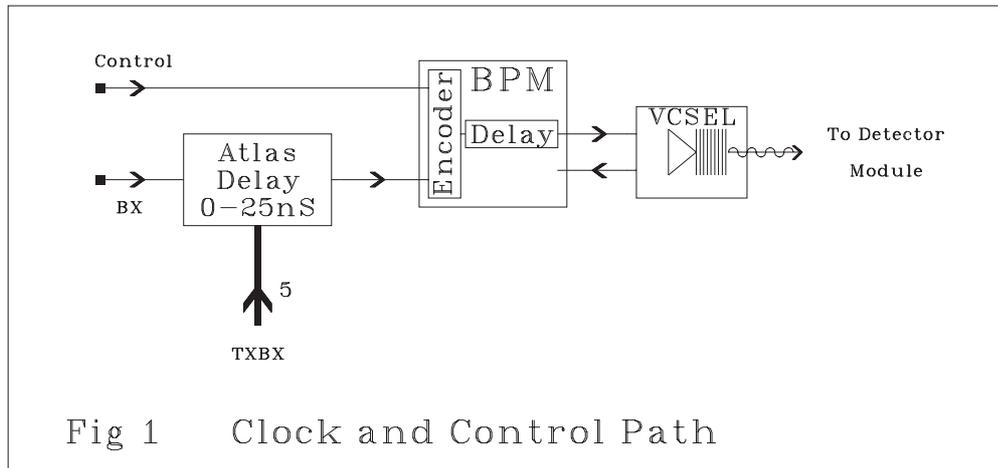
2.1.2. The BX signal has a phase trim of 0-25nS in 1nS steps to allow the BPM to strobe the control signals as soon as they are reliably valid, thus minimising the L1T latency.
