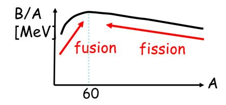
Most stable form of nuclear matter is at  $A\sim60$ . Expect a large amount of energy released in the FISSION of a heavy nucleus into two medium nuclei and in the FUSION of two light nuclei into a single medium nucleus.
