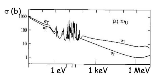
$\triangleright$  Hence, need to slow down fast neutrons before they escape or absorbed by  $(n,\gamma)$  process  $\rightarrow$  CHAIN REACTION
