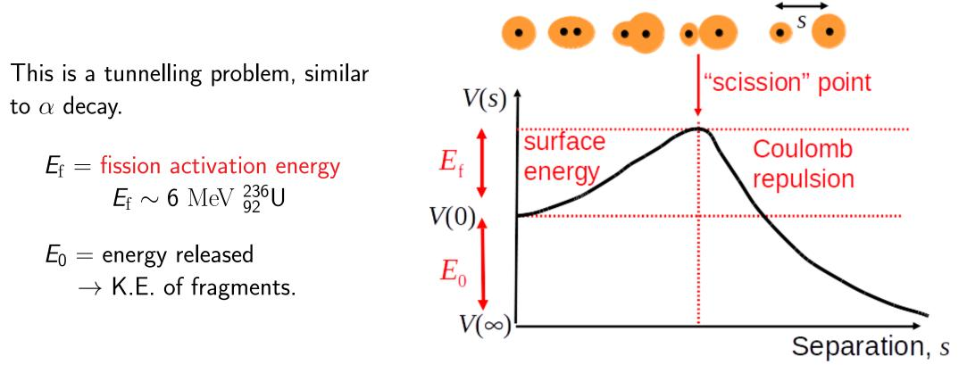
Although  $E_0$  is maximal for symmetric fission, so is the Coulomb barrier. In fact, asymmetric fission is the norm.
