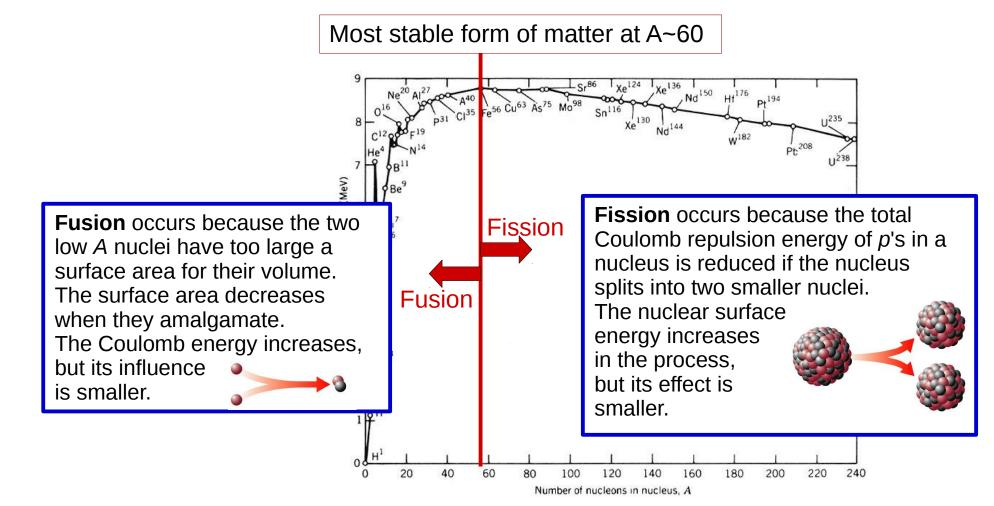
Expect a large amount of energy released in the fission of a heavy nucleus into two medium-sized nuclei or in the fusion of two light nuclei into a single medium nucleus.
