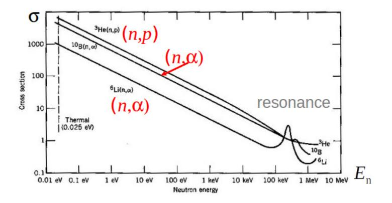
Low energy neutrons can have very large absorption cross-sections.
