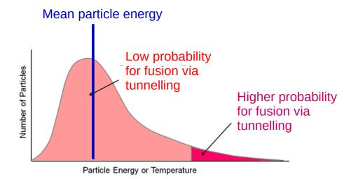
Reaction rate in unit volume for particles of velocity v:  $\Gamma = \sigma(v)\Phi N$ , where flux  $\Phi = Nv \sigma$  is dominated by the tunnelling probability  $P = e^{-2G(v)}$ and a factor  $1/v^2$  arising from the  $\lambda^2$  in the Breit-Wigner formula.
