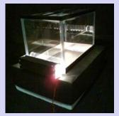
Our cloud chamber uses a tissue soaked in liquid isopropanol as a source of vapour.
