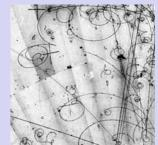
Charged particles like muons disturb the electrons and nuclei of atoms as they pass nearby and transfer a little of their energy as they do so.
