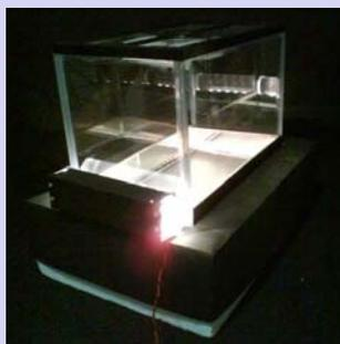
Our cloud chamber uses a tissue soaked in liquid isopropanol as a source of vapour.
