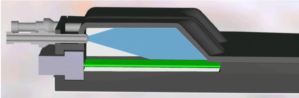
Light from calibration fibers illuminating ends of fibers from the scintillator where they are bundled
