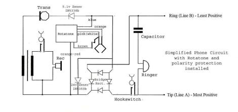
The above diagram shows the use of a bridge rectifier in order to make Rotatone polarity independent.
